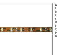
Model NO: CEGB3528-50 LED Power: 4.0-4.6W/m Input Voltage: DC12V Current: 330-385mA CCT: 2700K/4000K/6400K Beam angle: 120° Luminous flux: 250-300lm QTY/M: 60PCS/M Packing: 5M/Roll IP: IP20
