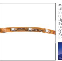
Model NO: CEGB5050R-50 LED Power: 6.12-6.84W/m Input Voltage: DC12V Current: 510-570mA Light Color: Beam angle: 120° Luminous flux: 135-160lm QTY/M: 60PCS/M Packing: 5M/Roll IP: IP20
